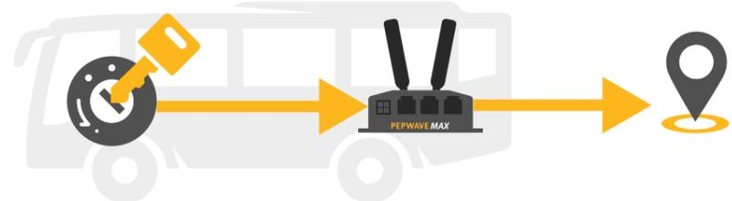
The MAX Transit Mini has specialized features for vehicular deployments. Ignition sensing, which detects the ignition status of the vehicle, enables the device to turn on and off as the vehicle starts up and shuts down. It is also equipped with GPS, enabling you to track its movements. With InControl's fleet management, you can review the route history of all your vehicles from any web browser.
