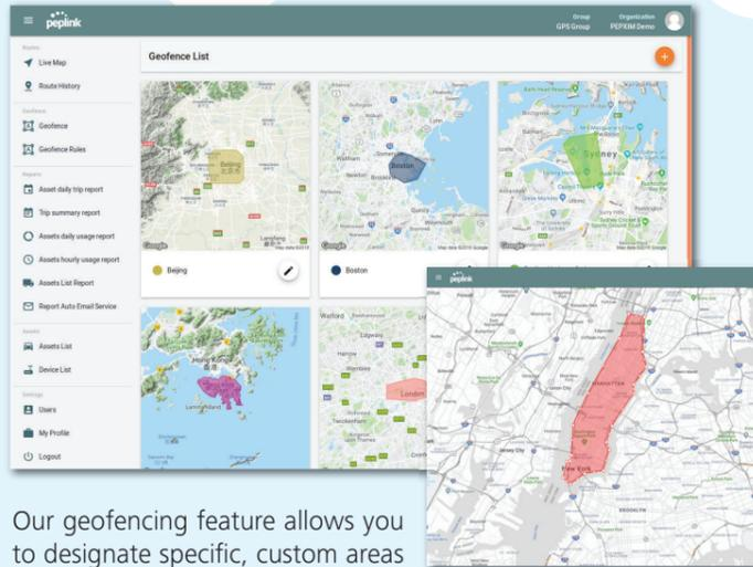
Our geofencing feature allows you to designate specific, custom areas on the map, and choose an action for the device to take when it moves into, or out of, any of these areas. For instance, a truck rental company that wishes to charge a certain rate for their vehicles being used in one area, and a different rate in another, will be able to not only see which area the vehicle is in, but also configure notifications for when the truck crosses from one area to another.
